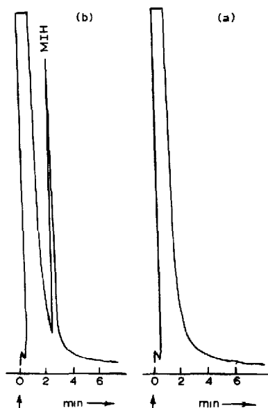
Fig. 2. Chromatograms of (a) solvent (ethyl acetate) and (b) 2 nmol of standard MIH. Retention time, 2.65 min; column, stainless-steel tubing (180 cm \times 2 mm I.D.) packed with 15% OV-225 coated on 100-120 mesh Chromosorb W HP; temperature, 220°C. Other conditions as described in the text.
